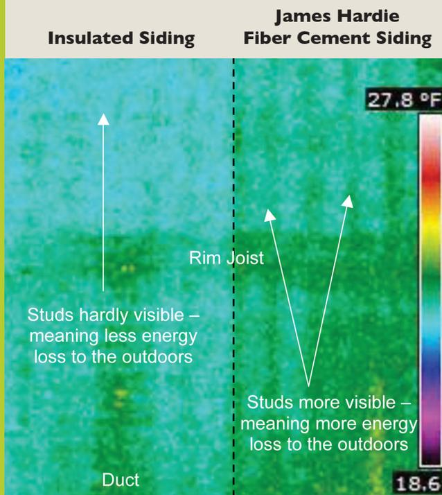
These thermal images from the NYSERDA study show how a home's studs allow heat to pass through a wall – a process known as thermal bridging. Insulated siding creates a barrier over the studs, interrupting the flow of heat.
